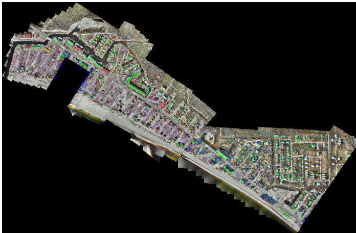
Figure: Predicted damage labels overlaid on the sUAS imagery.
